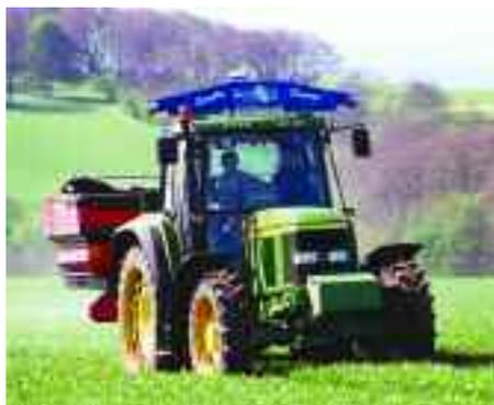
*The N-Sensor that first came to the UK in 1999 was a "coffin"-shaped box that sat on top of the tractor cab.*
